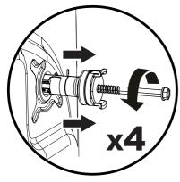
Transport screws should then be removed by pulling them out. The removed transport safety screws should be stored to be used again in case the machine needs to be transported again, e.g. if moving house.
