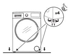
Do not install your machine on a carpet or such ground that will block ventilation from the base.
