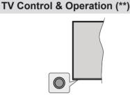
The control button allows you to control the Quick Standby-On functions of the TV.
