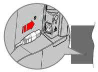
Plug one end (the two-hole plug) of the supplied detachable power cord into the power cord inlet on the rear side of the TV as shown above. Then plug the other end of the power cord into the mains socket outlet. The TV will switch on automatically.
