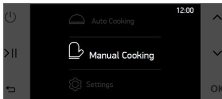
In the manual cooking menu, cooking functions, temperature, boost function, cooking duration and cooking end time can be set by end user. To change any specification, navigate with UP & DOWN buttons and select the specification with OK button. After tapping, selected specification blinks. While blinking, UP & DOWN buttons are used to change the value of the specification. You can finalize the selection by tapping OK button.
